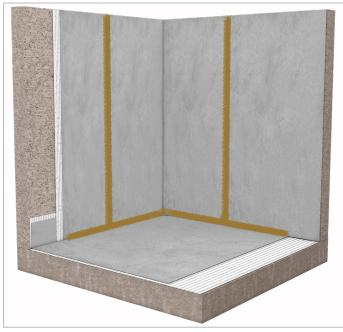
3. Apply a thin layer of C2 S1/S2 tile adhesive using a 4 mm notched trowel and cover the wall with **ECODRY50** membrane, leaving an overlap between membranes of at least 5 cm. Press the membrane firmly onto the structure with the help of the trowel, making sure to remove all possible air pockets that may have appeared. Seal the joints with **SEALPLUS** by double sealing (see point 2.).
