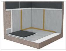
3. Spread C2 S1/S2 tile adhesive with the 4/6 mm notched trowel and cover the wall with the ECODRY50 membrane leaving an overlap between membranes at least 5 cm. Check that the membrane is well extended, with the help of the trowel, remove any air that may have been generated. Seal the joints with **SEALPLUS** making a double seal (see point 2). Proceed to floor covering and walls.
